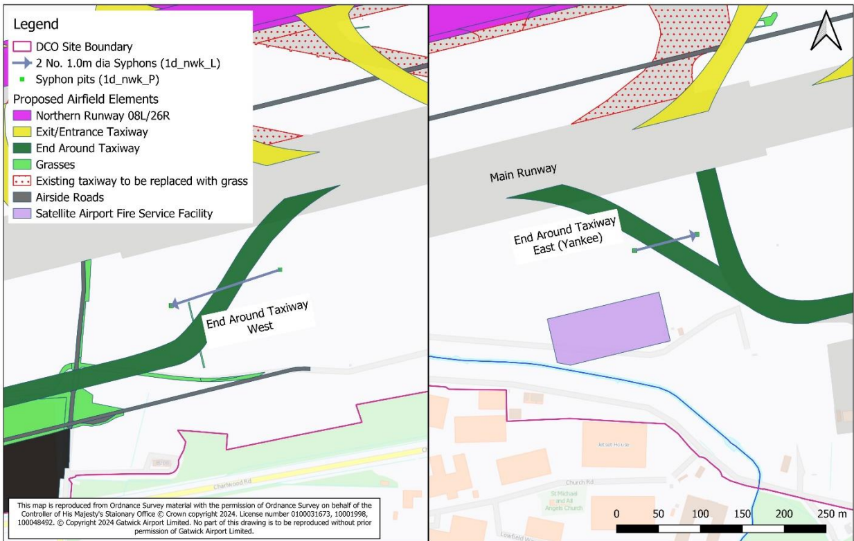
Figure 6-17: End Around Taxiway West and End Around Taxiway East (Yankee) Syphons.
